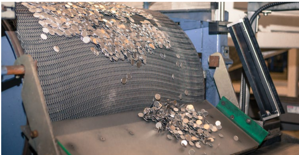
Blank production using the Mint's multi-ply plated steel (MPPS) technology greatly reduces dependency on expensive base metals.
