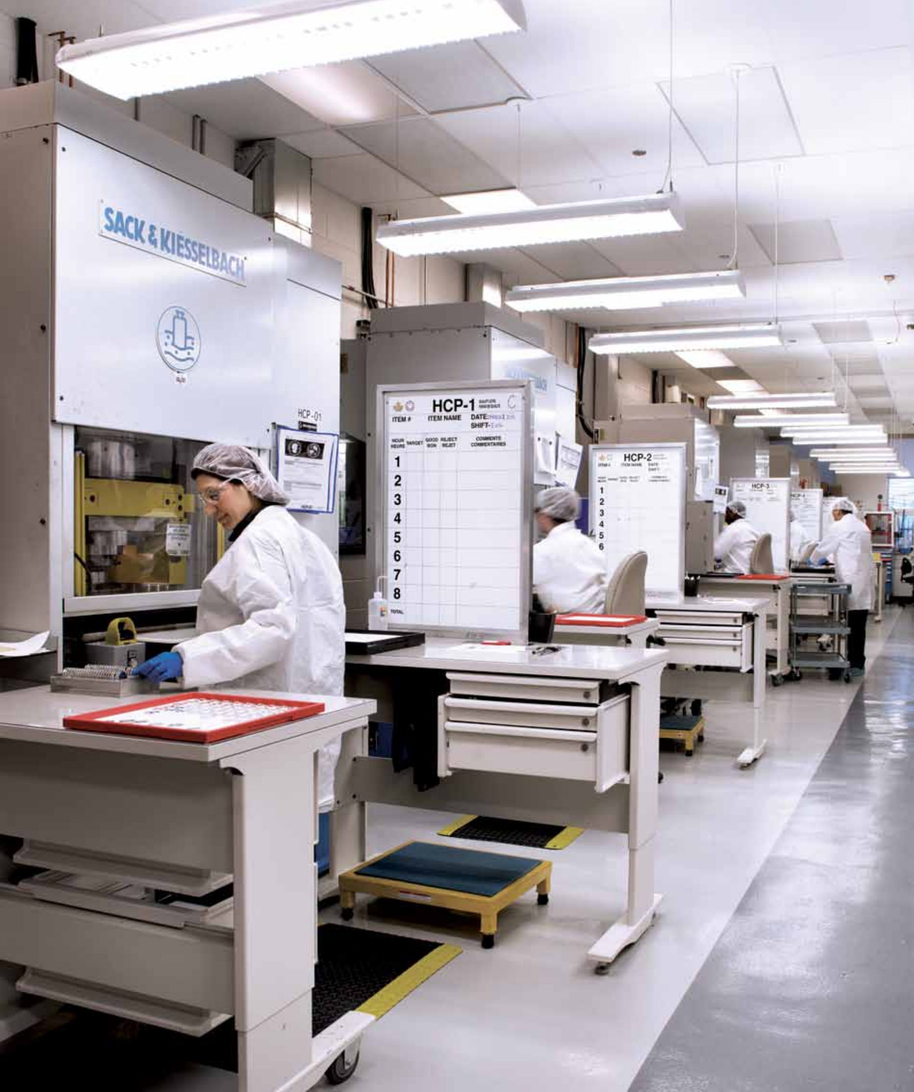
The Mint acquired three additional Sack & Kiesselbach coining presses to prepare for growth and meet production requirements ahead of Canada's 150th anniversary celebrations in 2017. One of these includes an automatic feeding system that will bring greater efficiency and quality to numismatic production while mitigating the risk of repetitive strain injuries.
